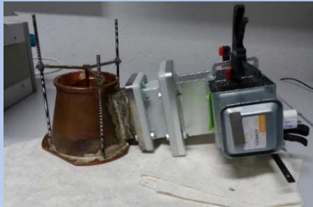
M. Tajmar's prototype with Waveguide, Magnetron 2015
