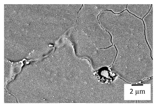
Liquation of carbides causing intergranular crack in HAZ of SHT+AGED condition
