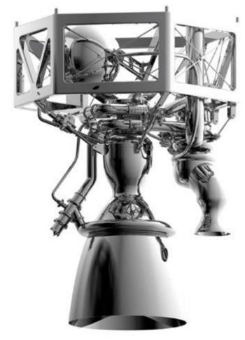
Prometheus, a low cost reusable rocket engine, using methane propellants
