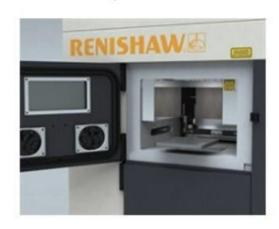
Build plate is loaded into the system chamber and secured.
