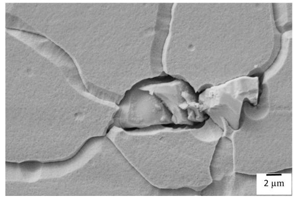
Liquation of carbides creating crack in HAZ of wrought Alloy 718
