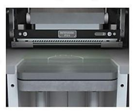
Build plate moves down and next layer is built up.
