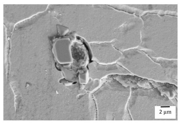
Liquation of carbide and Laves phase causing intergranular cracks in SHT condition
