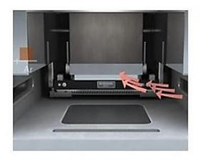
Chamber is filled with argon iner gas - class leading low gas consumption.
