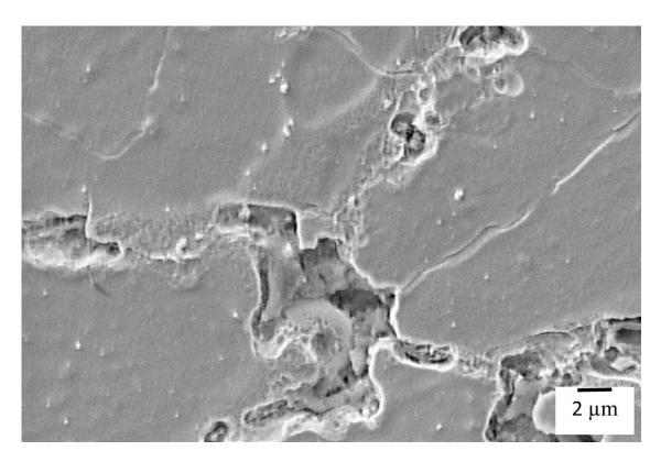
Cracking in as-built condition due to the liquation of Laves phase and carbide
