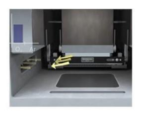
Build chamber is prepared with vacuum removal of air.
