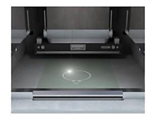
Laser melting using a fibre laser.
