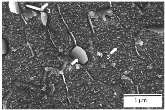
Microstructure of SHT+AGE condition showing (1) delta phase, (2) MC-type carbide and (3) matrix with strengthening phases  $\gamma'$  and  $\gamma''$
