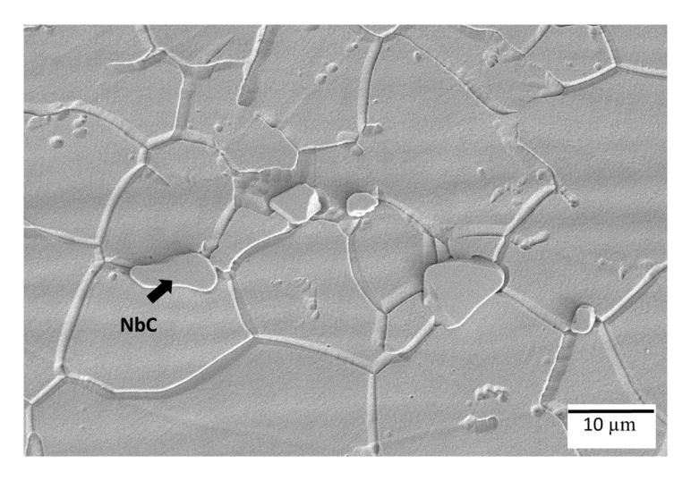
Mill-annealed at 982°C - 4.5min
