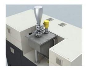
Loading metal powder before and during build.
