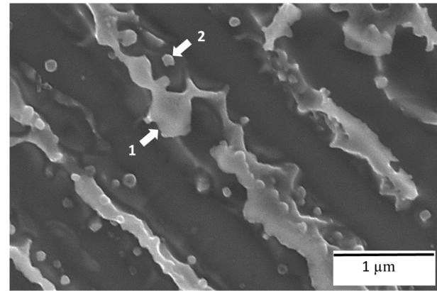
Interdendritic regions in as-built condition showing (1) Laves phase and (2) MC-type carbide
