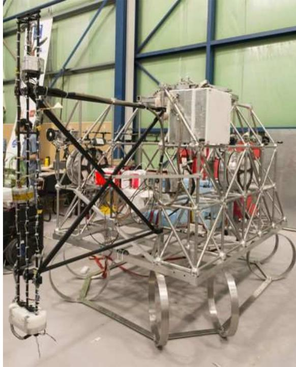
**CNES Helios payload gondola**
