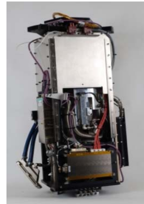
Isothermal solidification experiment furnace, using X-ray source as diagnostic system
