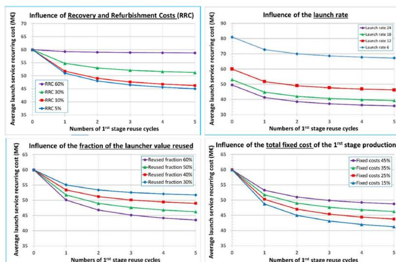
Figure 1: Results of a parametric study of launch service costs using reusable vehicles by CNES [2]
